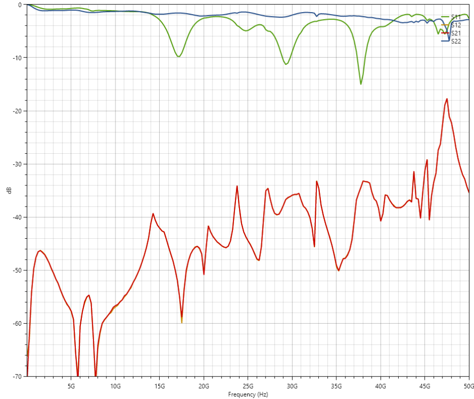
Figure-33 5G Band SP3T Switch Inside Module Measurement When Port-2 is Off State
