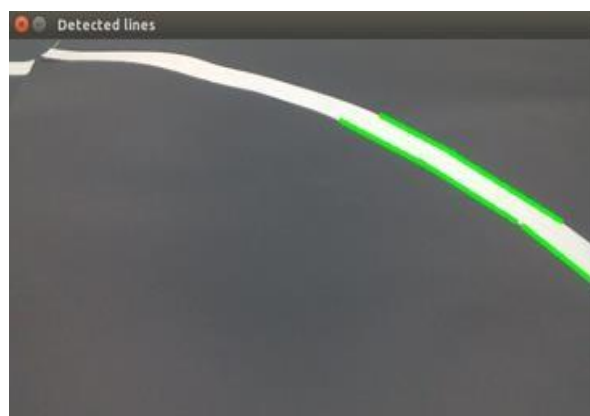
Figure -3: Houghline of the turning left
