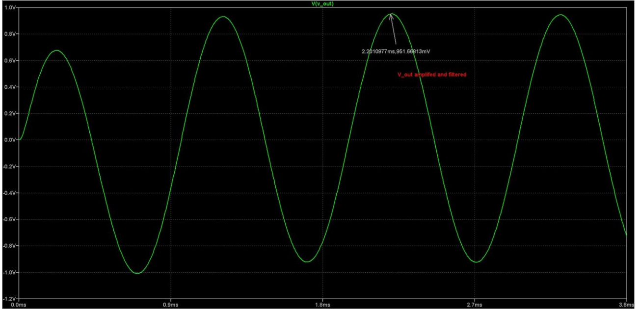
Figure 19. Filtered and amplified output time domain signal
